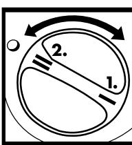
To change from one gear to the other, turn the gear selection lever through 180°.
